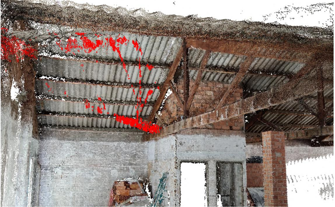
Figure 6.1: An example of reconstruction error produced by Metashape in site BCN1. The truss in red does not in fact exist.
