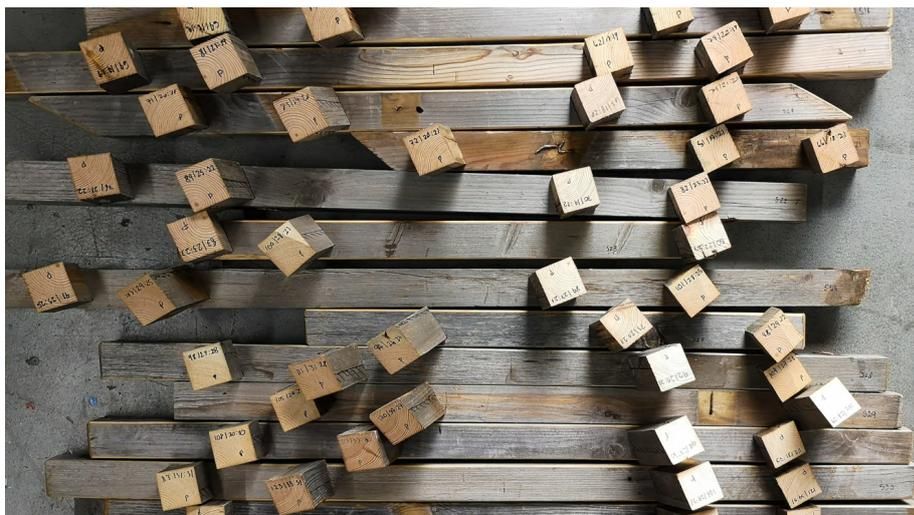
Figure 4.13: Stock of pre-assembled secondary-layer components
