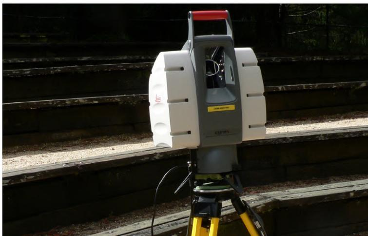
Figure 5.1: An accurate but expensive mounted LIDAR model
