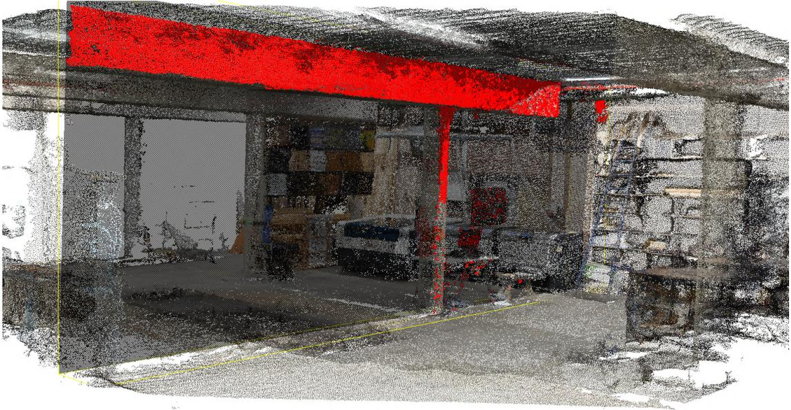
Figure 2.5: In site IAAC1, RANSAC has correctly extracted one face of the concrete beam, but has assumed part of the adjoining column, as well as some clutter elements, to be part of the plane
