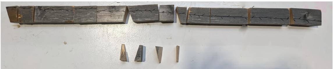
Figure 4.16: Stock of connectors cut from a single input element, with minimal waste chips
