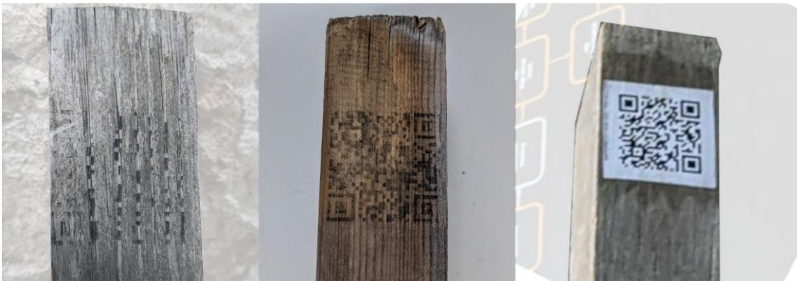
Figure 3.12: Test pieces using ink transfer, laser etching, and paper tags
