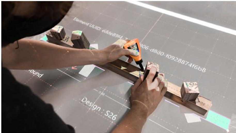
Figure 4.12: Pre-glueing connectors for all secondary-layer structure components
