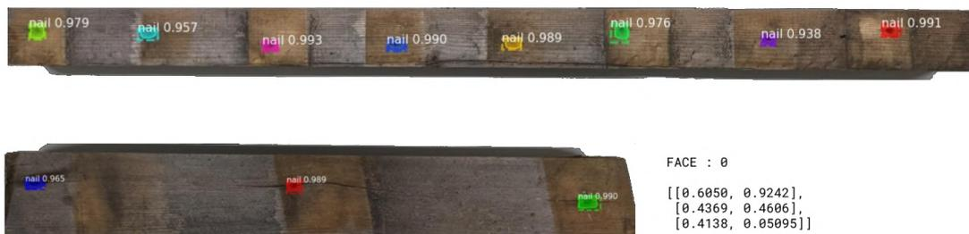
Figure 3.8: Example output when localizing texture defects using Mask R-CNN
