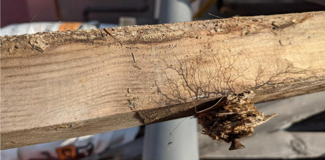
Figure 4.2: An unprocessed recovered element showing remaining decayed plywood base and wood screw connector
